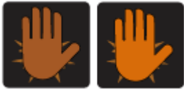
A flashing hand or flashing DON'T WALK sign
